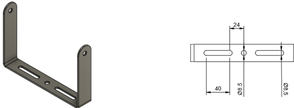
Figure 2 U-Bracket mounting holes.
